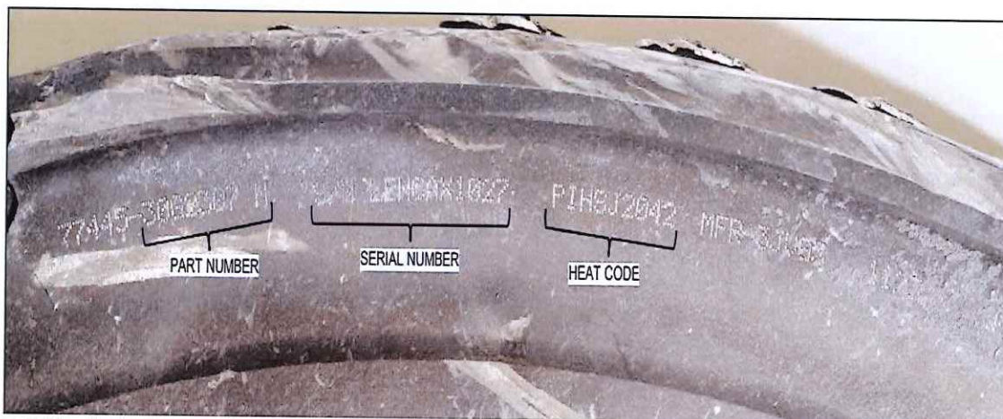
Fig. 1.16.1.a. High Pressure Compressor (HPC) 7 th Stage Integrally Bladed Rotor (IBR-7) recovered part identification.
