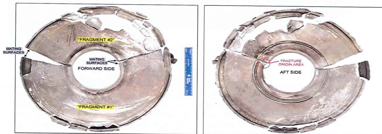
1.16.3.1.a. Overall views of fragments and fracture radially from bore to rim in two places spaced ~220 degrees apart.
