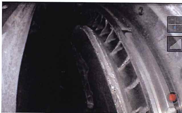
Fig. 1.3.a. High Pressure Compressor [HPC] 7th Stage Integrally Bladed Rotor [IBR-7].
