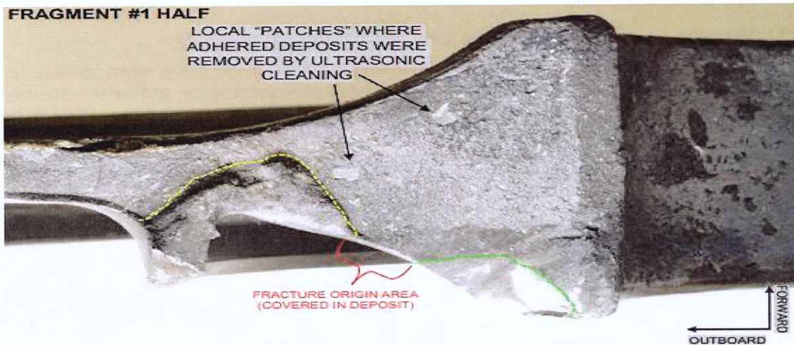
Fig. 1.16.3.2.b. Fragment #1 fracture half at bore region.
