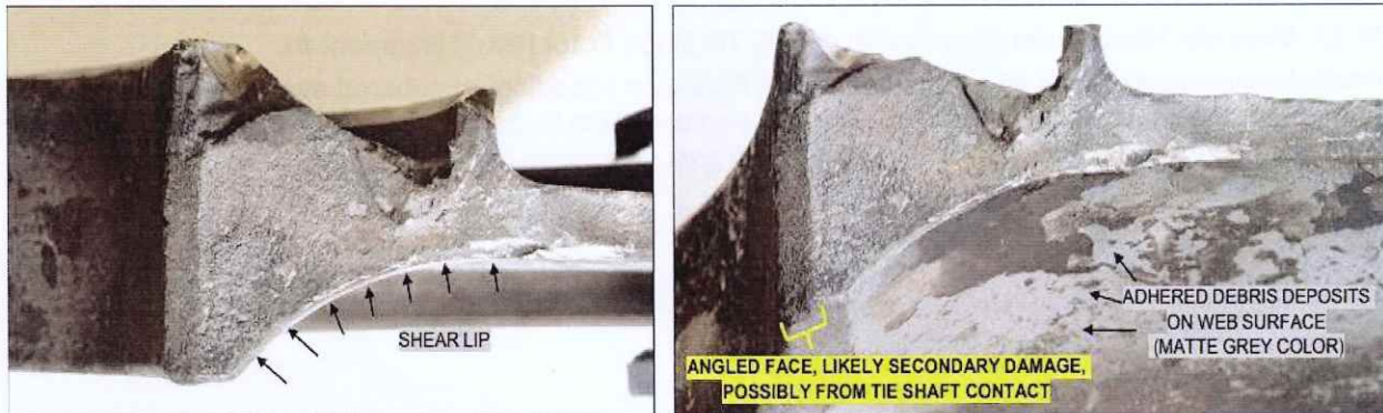
Fig. 1.16.3.2.c. Fragment #1 primary radial fracture surface was covered in a layer of debris that obscured fracture & angled face likely secondary damage.
