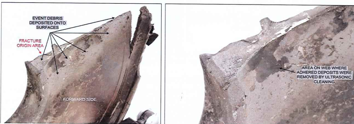
Fig. 1.16.3.2.a. Fragment #1 surface showing a thick layer [cladding] of adhered event debris deposits on the forward web/bore surfaces adjacent to the fracture.
