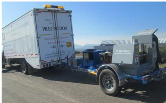
*Figura 5. DEFLECTÓMETRO DE IMPACTO DYNATEST (HWD)*
